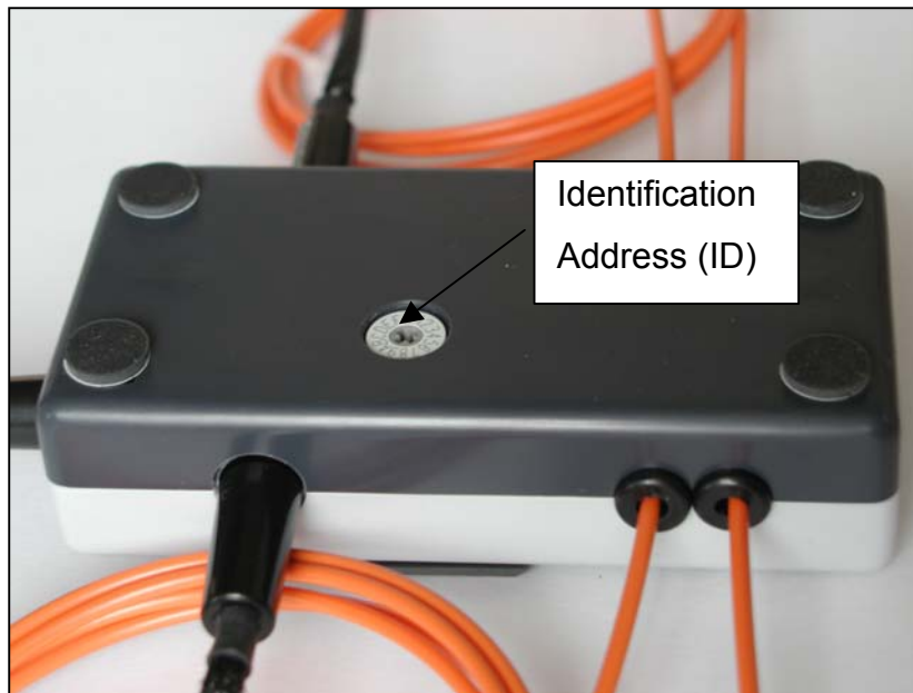
Figure 6: Address switch on the bottom side
