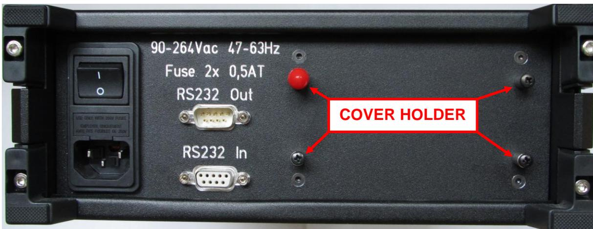
Figure 3: Rear panel view to the cover holder
